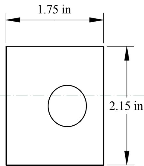
Welded tab with mounting hole to pick up bolt from crossmember
